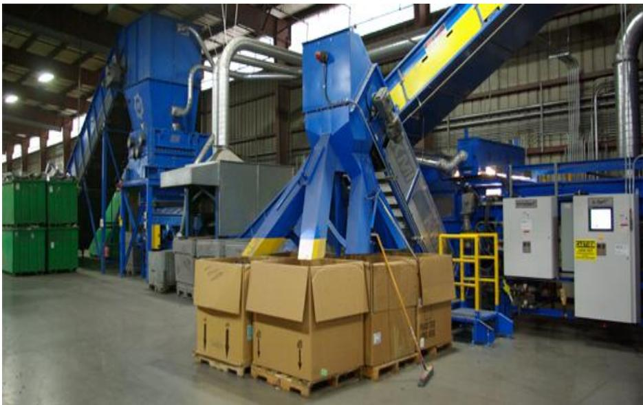
The materials being recovered are largely ferrous metals, aluminum, copper, circuit boards as well as the plastics ABS, HIPS, PC and ABS-PC.
